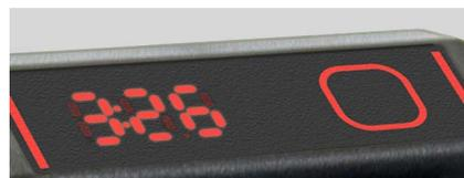
A single button press shows individual battery capacity as a percentage, in 1% increments. The display maintains accuracy by tracking cell-performance and adjusting calibration values to compensate for cell-aging.
