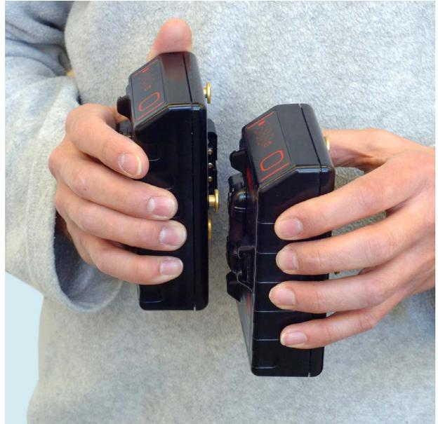
*Linking two PL150 batteries produces a capacity of 300Wh, ideal for digital cinema applications.*
