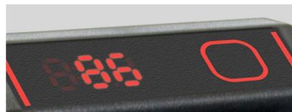
PAGlink batteries display their remaining capacity in the camera viewfinder/LCD by communicating automatically with the data system that also allows Anton/Bauer batteries to display capacity.
