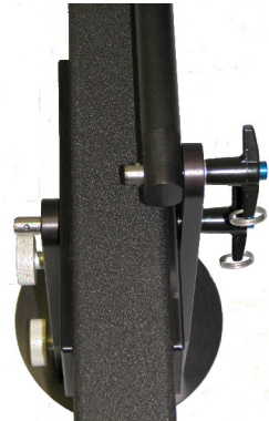
Fulcrum from above note parallel rod and connector pin placement
