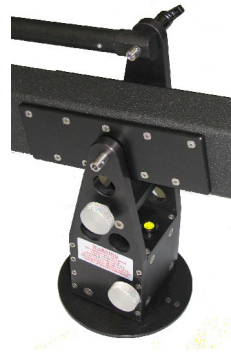
Assembled fulcrum Top knob: tilt brake Bottom knob: pan brake
