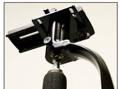
6. **Vertical Balance** - Now you can check the vertical balance of the FlowPod to see if you need to add, remove, or adjust the position of the counterweights. Use as few weights as possible, and start with the weights at the top of the shaft. When vertically balanced, the FlowPod should not lean or sway when moved around.
